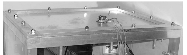
FIG. 3. Photography of the experimental setup with the primary shaker below the plate in the background and the inertial actuator above the plate in the foreground.
